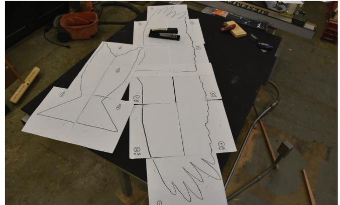
Once the schematics are laid out and fit onto the mat, staple the paper to the mat by locating the staples on the inside of the body/wings outlines as the outside paper will be cut away.
