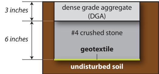
**Figure 2.** Construction details for heavy use area pads.
